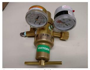
FIGURE 3 HIGH PRESSURE (HP) ADJUSTABLE REGULATOR
