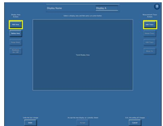
3. Select **Add Trace** to add parameters to an area. For each trace, choose a measurement from the available list. For EEG waveforms, CSAs and DSAs, select an EEG channel from the montage associated with the protocol.
